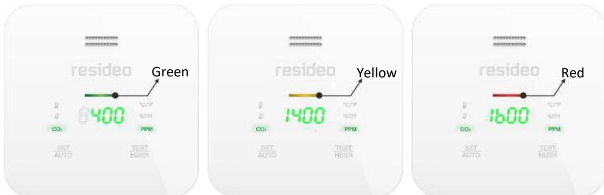
When CO<sub>2</sub> concentration is  $\leq 1000\text{PPM}$ , the status indicator turns green.
