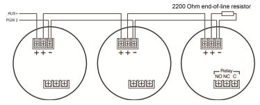
Figure 2-16 2-Wire Smoke Detector Wiring
