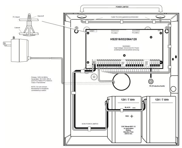
Figure 2-1 Wiring Routing (North America only)
