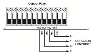
Figure 2-6 HSM2HOSTx Wiring Diagram
