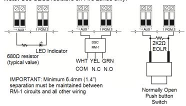
Figure 2-12 LED Output with Current Limiting Resistor and Optional Relay Driver Output.
