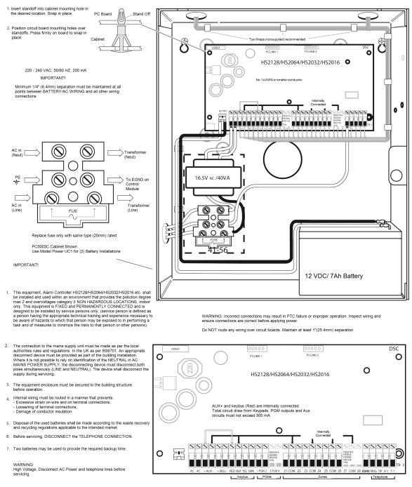
Figure 2-2 Wiring Routing (EN50131 only)
