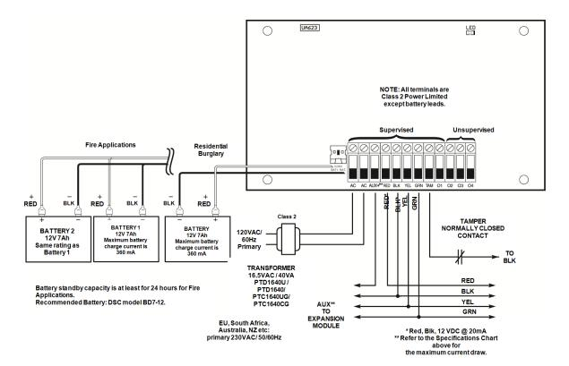
Figure 2-7 Power Supply Wiring
