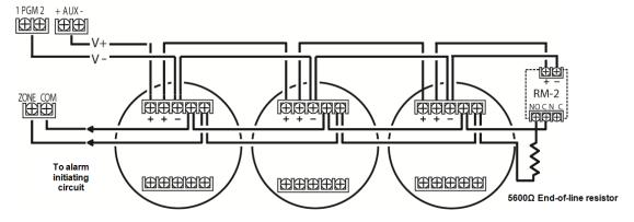
Figure 2-15 Smoke Detector Wiring
