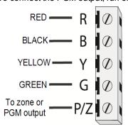
Figure 2-8 Keypad P/Z Terminals
