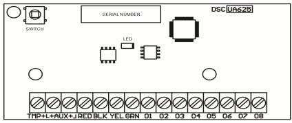
Figure 2-5 HSM2208 Output Expander
