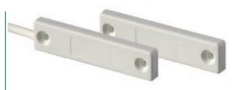
The reed part contains the reed encapsulated watertight with the two-component polyurethane resin in conjunction with a loop tamper in order to reduce the risk of burglary.
