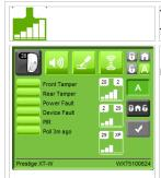
The device signal strength meter details the strength of signal between the device and the receiver, or the device and another device on the system which it is hopping through.
