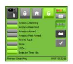
SmartKey™ switched on showing full details of the SmartKey™ settings and system status
