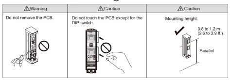
Keep the detector parallel to the ground. Consider the direction of the intruder, for the setting of the detection area. Install the detector in a place where it is free from false alarm factors. For example: • Sunlight and reflection • Heat source • Heat source • Diplots moving in the wind • Objects moving in the wind • Objects
