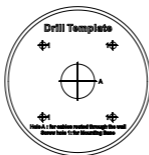
Figure 2-12 Drill Template of the Junction Box
