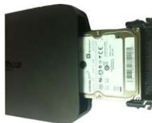
③ Put the HDD into the device
