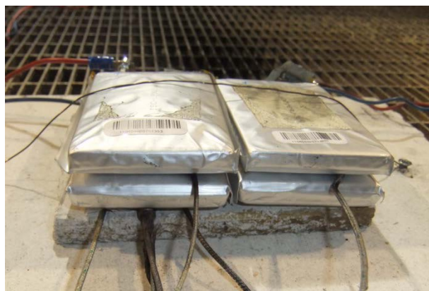
Figure 6: Set-up for fire extinguisher test for 2x2s1p configuration, below left cell is the heating rod
