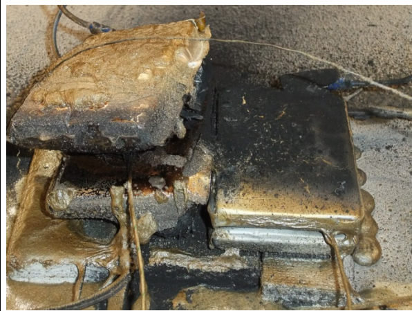
Figure 12: Cells after test rear view
