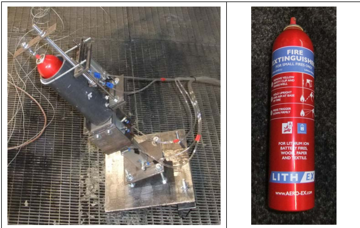
Figure 4: 400 ml Aerosol fire extinguisher filled with AVD and pressurized operated with pneumatic manipulators
