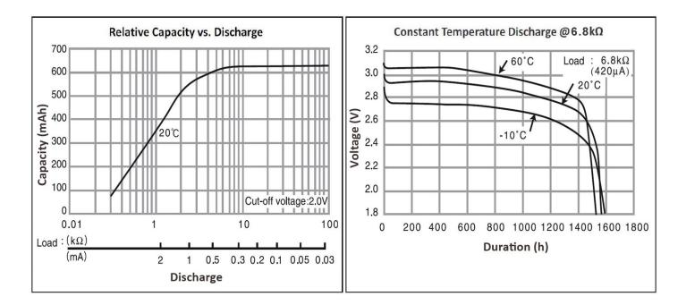
\* Nominal capacity indicates duration until the voltage drops down to 2.0V when discharged at a nominal discharge current at 20°C. \*\* When using these batteries at temperatures outside the range of -20 to +60°C, please consult Duracell in advance for conditions of use.
