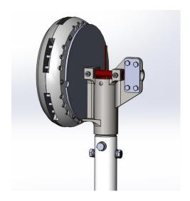
• Install the blades to the generator with 18pcs of bolts (M6\*28).
