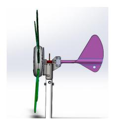
Fasten the gyrator front cover to the back cover via 3pcs of bolts (M5\*10).
